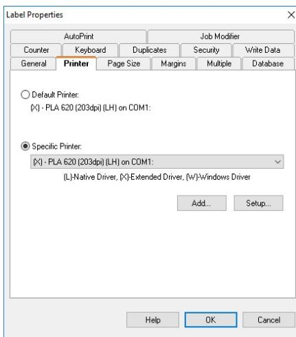
**Figure 2-13** Printer Tab
