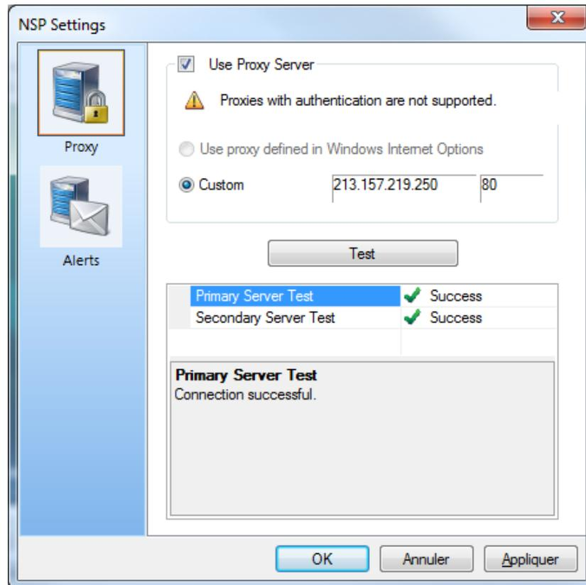
4. Check **Use Proxy Server**. Define the valid IP address of your proxy server in the **Custom** field and click the **Test** button to test your connection.
