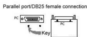
If you need to use a printer on the same parallel port, simply plug it into the software protection key. It may be necessary to turn the printer on in order for the software protection key to be recognized.
