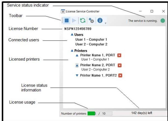
图 5: Main Service Control window for licenses limited by printers
