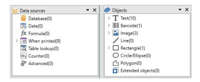
The up and down arrow keys on your keyboard allow you to move up and down the object tree. The + and - symbols allow you to expand or shrink the list and display the list of variables associated with each data source or the objects available for each category.
